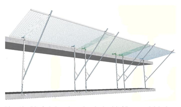
Prior to Visor T Evo fan in the market, we have developed the full system and obviously we get the certification. The certification is made according to European Standard EN 1263.1 in exclusively all the parts shown in this Standard.
